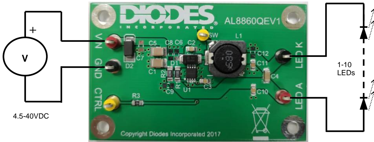
Figure 1: AL8860QEV1 evaluation board and connection diagram
