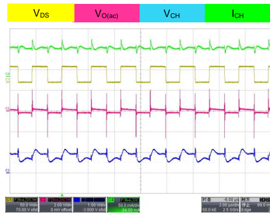
PWM to Analog Dimming ( f_{PWA} = 10\text{kHz} , 50% Duty)
