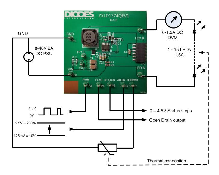
Fig. 1 ZXLD1374QEV1 Evaluation board connection diagram
