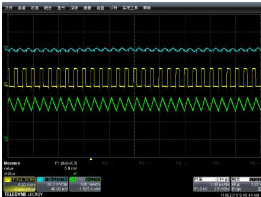
Operation waveform at Iout=1A (Blue-VoutAC; Yellow-Vsw; Green-IL)
