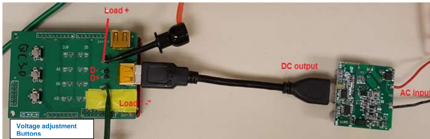
Figure 10: The Test Kit Input & Output and E-load Connections
