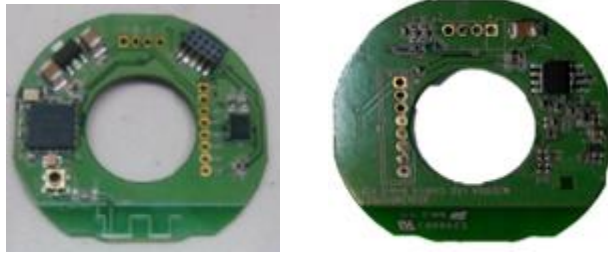
Figure 5 - Wireless & LED Driver Board (41.2mm Outside Ring, 18mm Inside Ring)
